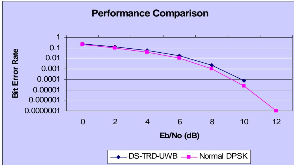
Figure 6. Simulation and Ideal TRD Performance Comparison.
