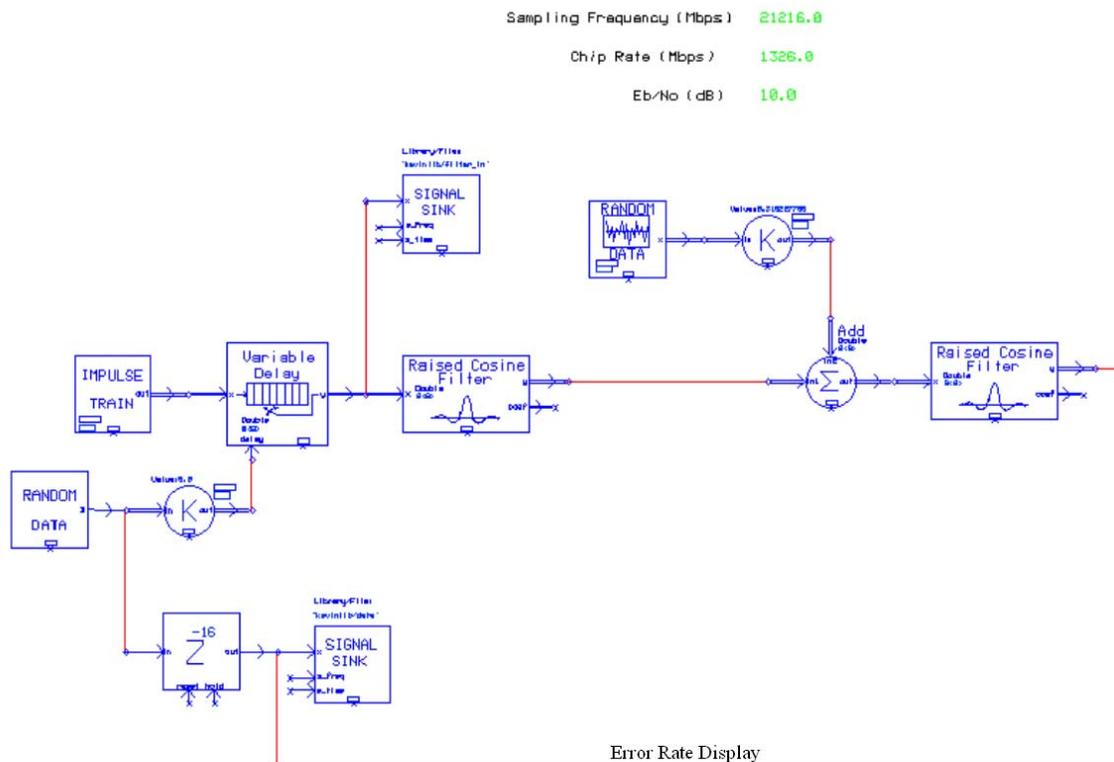
**Figure 2. Simulation System – PPM Transmitter.**
