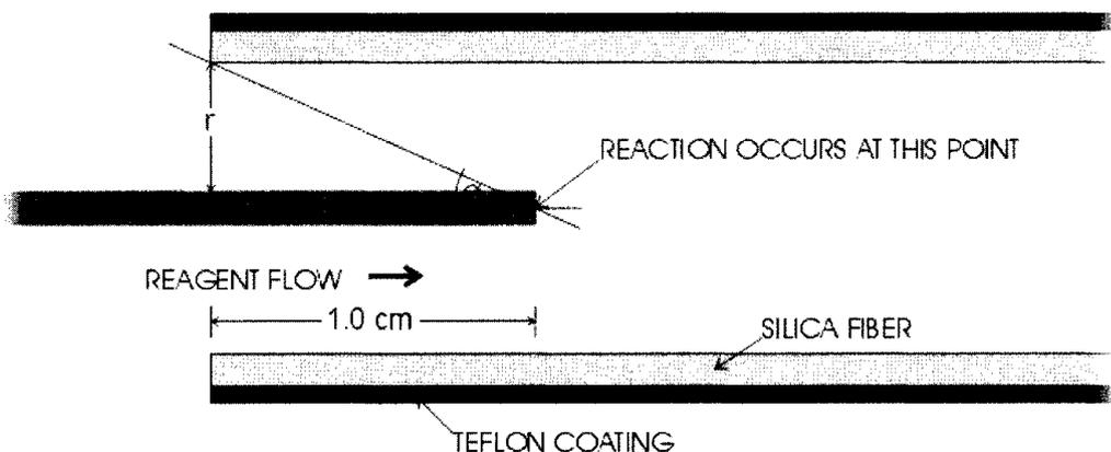
**Figure 13. Angle between silica fiber and tubing.**
