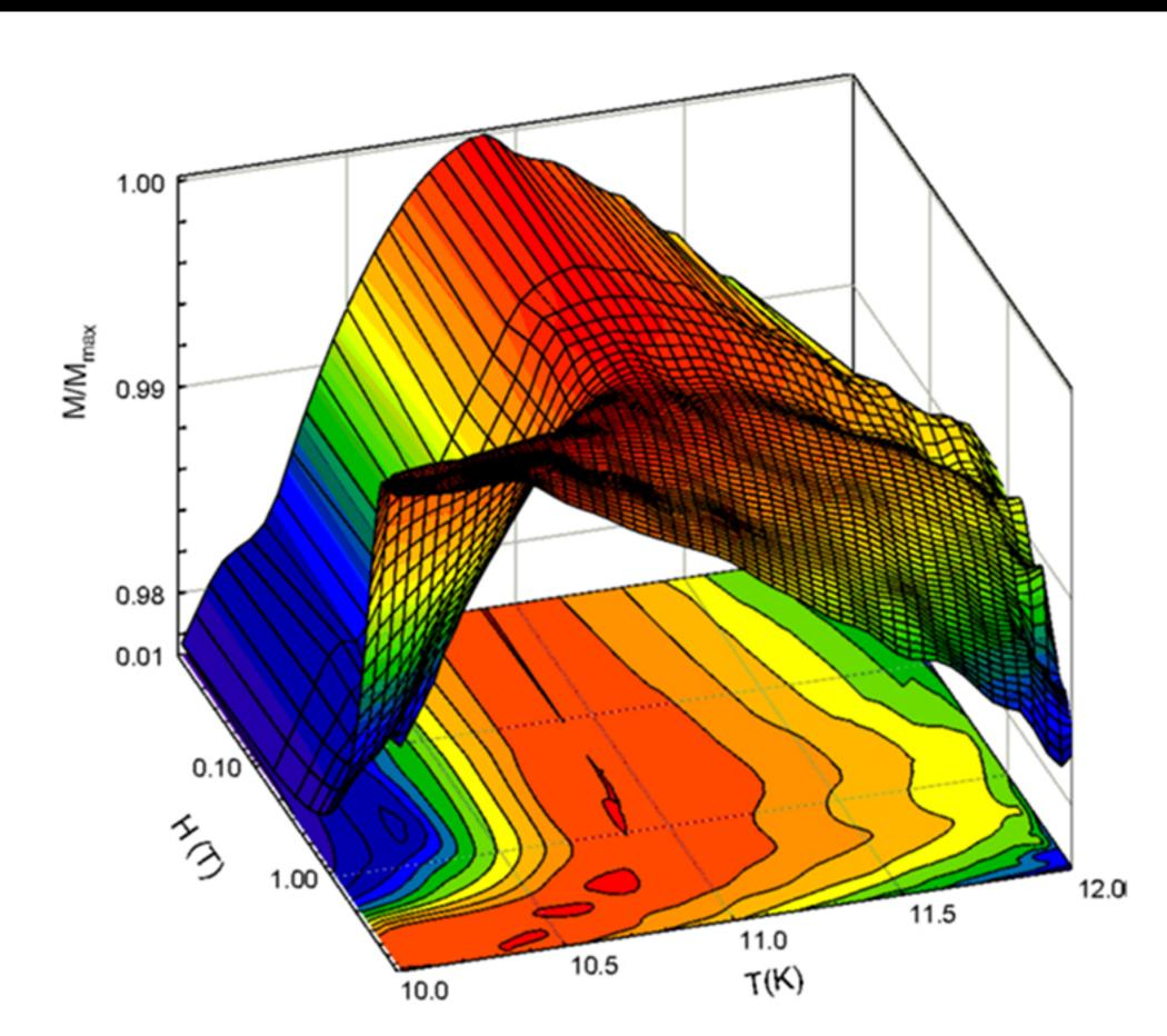
Normalized magnetization versus temperature and field for  $Ga_{0.91}Mn_{0.09}Se$ . Note the log scale on the H(T) axis. The critical temperature  $T_c$  at 11.2 K is just above the 10.9 K cusp at low fields. Above  $T_c$ , the spin-glass exhibits paramagnetism. Below the  $T_c$ , the magnetization exhibits behavior that suggests that a spin-glass transition is taking place.
