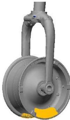
**Figure 15: Bead seat pressure caused by vertical force**
