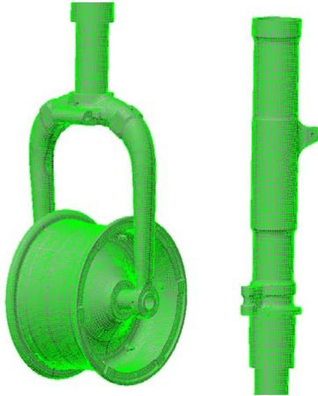
**Figure 19: Nose gear mesh**
