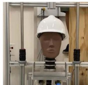
Fig. 4: Head Form model with Control Helmet<sup>3</sup>
