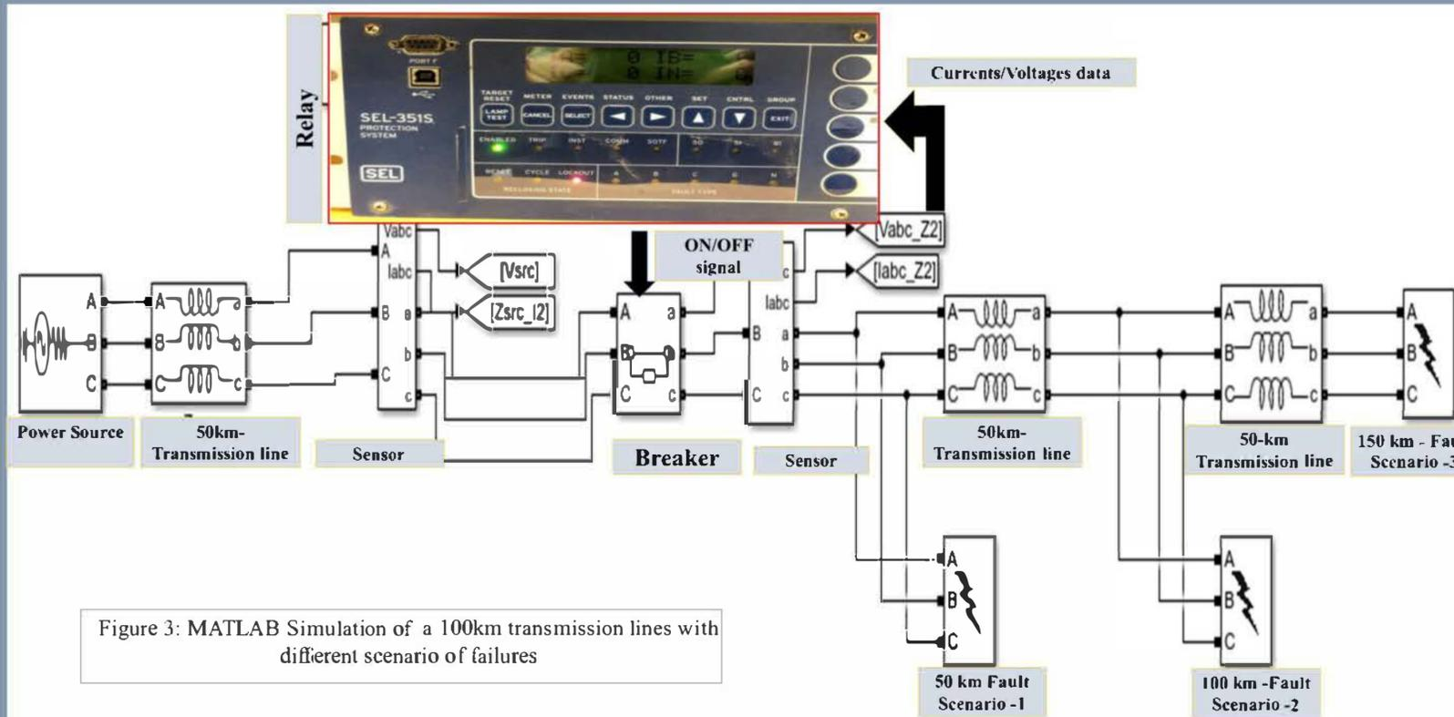
Figure 3: MATLAB Simulation of a 100km transmission lines with different scenario of failures
