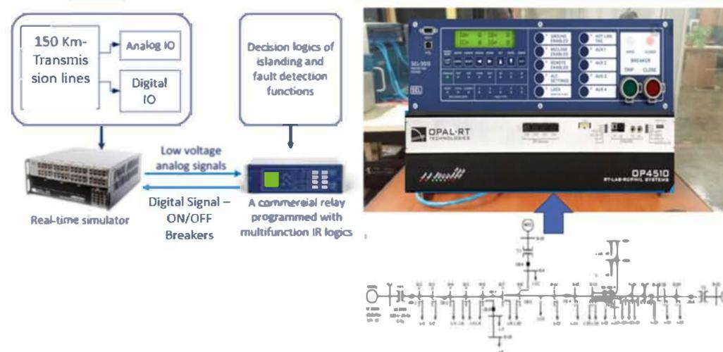
Figure 1: Hardware-In-the-Loop (HIL) testing platform
