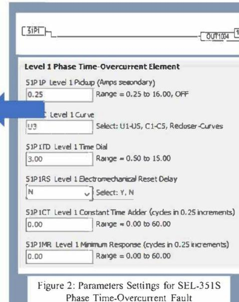
Figure 2: Parameters Settings for SEL-351S Phase Time-Overcurrent Fault
