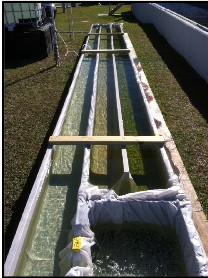
Figure 30 - Algal Growth in Contact Chamber
