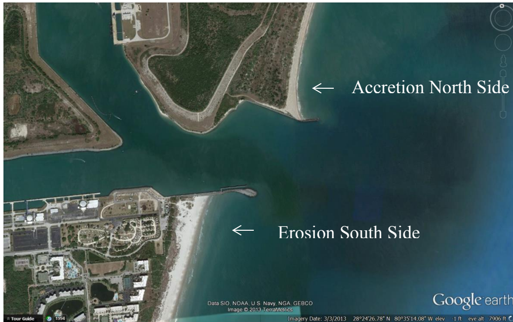
Figure 1.1: Entrance to Port Canaveral, Florida, showing accretion on the updrift (north) side and erosion on the downdrift (south) side as commonly occurs at jettied inlets on Florida's east coast.
