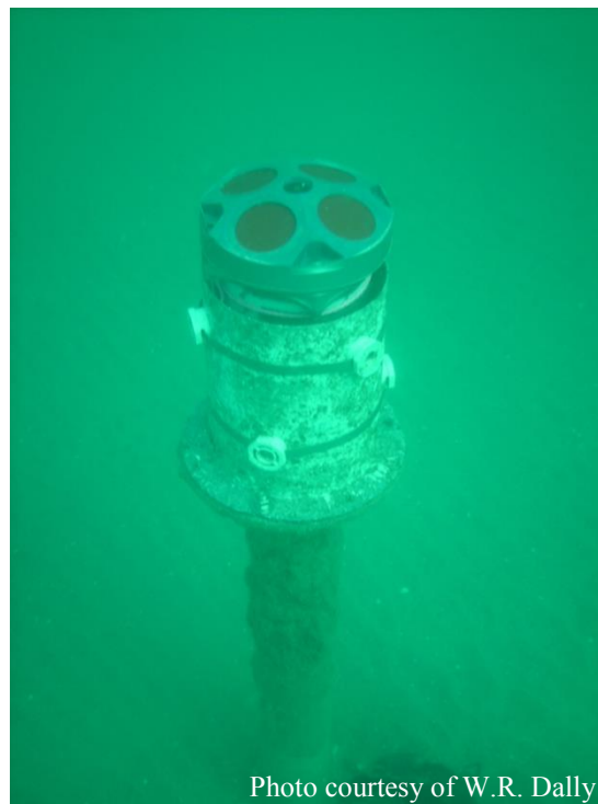
Figure 1.6: ADCP attached to the jettied spud at Spessard
