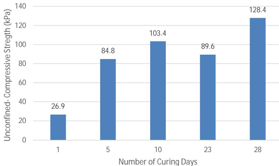
Figure 4.6 Results for unconfined compression testing Mix 2
