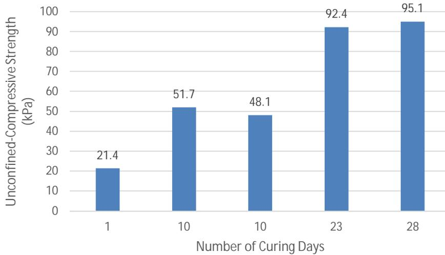
Figure 4.5 Results for unconfined compression testing Mix 1
