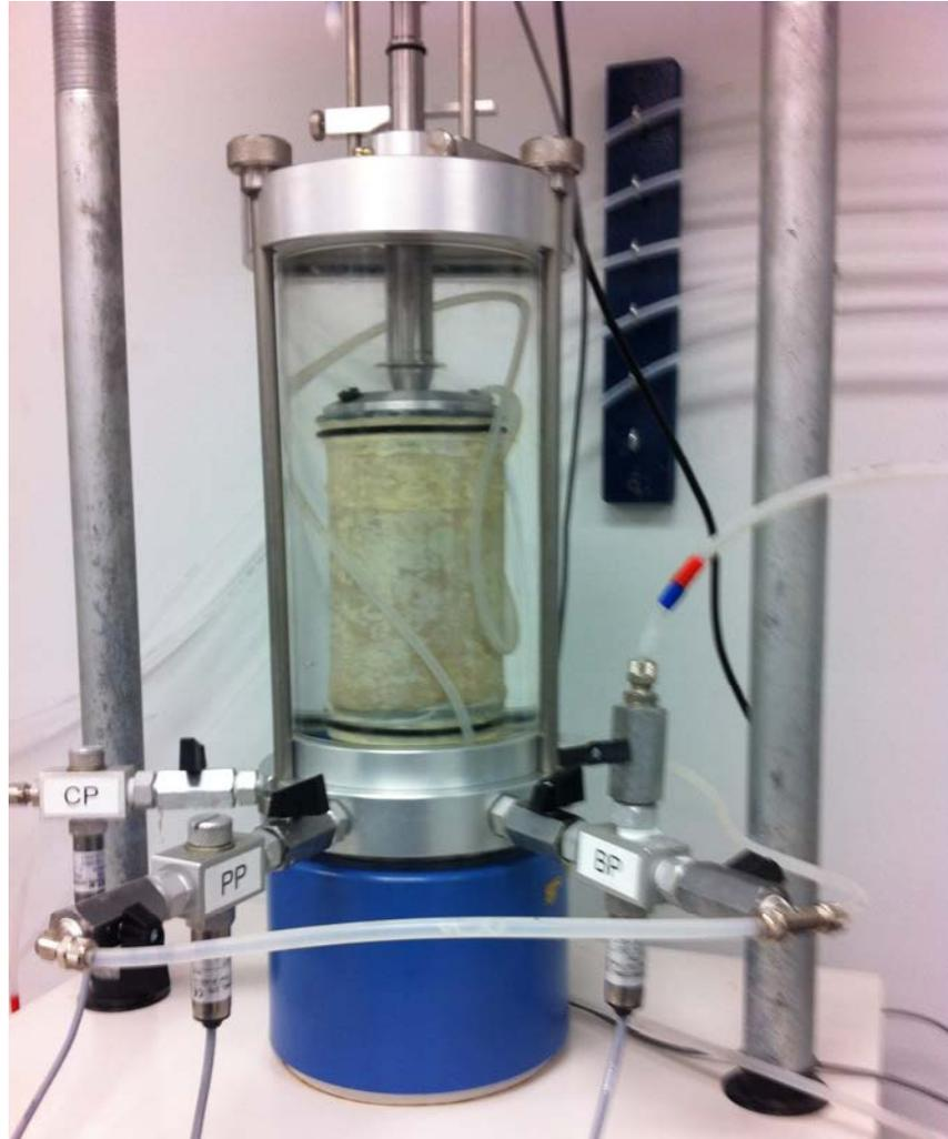
Figure 3.6. Triaxial cell placed on the load frame
