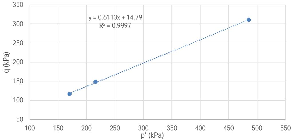
Figure 4.3 p'-q graph for consolidated undrained Mix 1 twenty eight day curing
