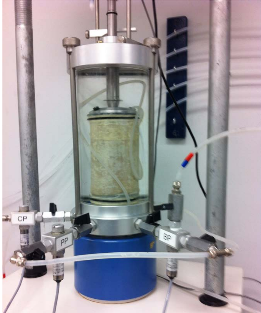
Figure 3.6. Triaxial cell placed on the load frame
