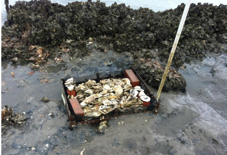
Figure 1-4 Deployed plastic settlement tray behind one section of the artificial reef installed along the Guana Peninsula in the Guana Tolomato Matanzas National Estuarine Research Reserve, Florida, U.S.A. Trays contained one layer of oyster shell ( Crassostrea virginica ) as well as four bricks for stabilization. They were deployed behind reefs (natural and artificial) as well as 3 m in front of fiber logs and at approximately the same elevation within an unstructured site.
