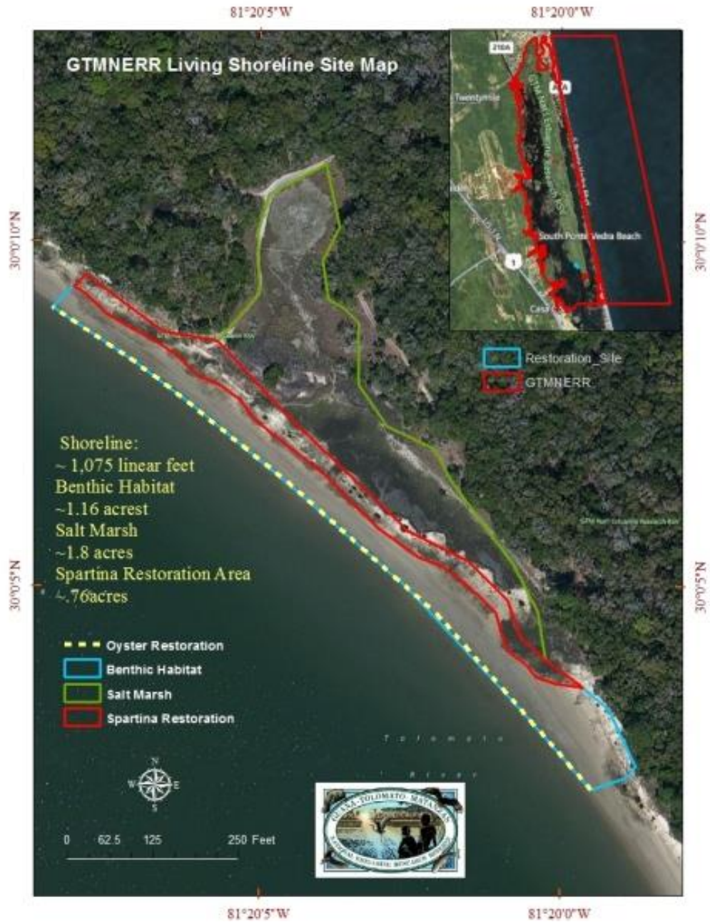
Figure I-1 Map of oyster restoration along Wright’s Landing in the northern Guana Tolomato Matanzas National Estuarine Research Reserve (GTM NERR). Wright's Landing is along the eastern shoreline of the Tolomato River on th Guana peninsula. Fiber logs were installed within the Benthic habitat 5m from the marsh edge in addition to 100-m north of the reef along the same shoreline. Source: Friends of the GTM Reserve http://gtmnerr.org/Oyster-Reef-Restoration-Project.php
