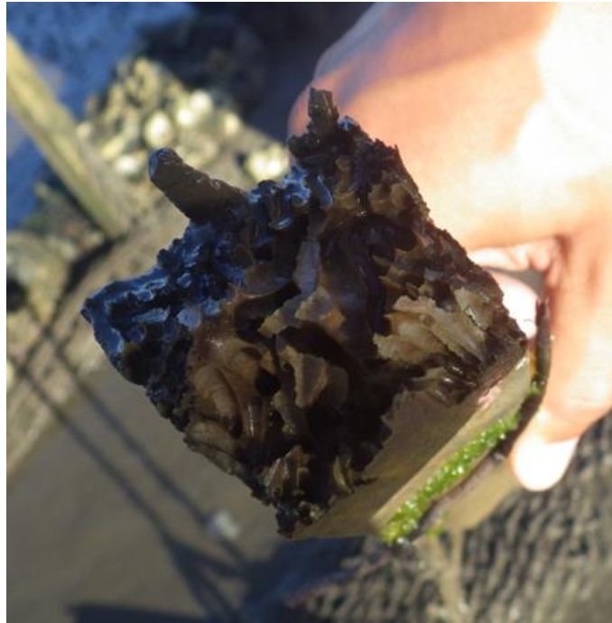
Figure I-6 Evidence of shipworm ( Teredo sp.) colonization of the wooden stakes securing all the fiber logs installed within the artificial oyster reef as the combination living shoreline treatment along Wright's Landing in the northern Guana Tolomato Matanzas National Estuarine Research Reserve. Photo was taken July 15, 2014 after the installation of the fiber log only treatment was installed 100-m north of the artificial oyster reef.
