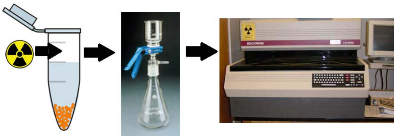
Figure 4. Basic protocol for a radioactive isotope experiment using brush border membrane vesicles. Radioactive ^{14}\text{C} -sucrose ( 3\ \mu\text{l} ) was added to the incubation medium ( 140\ \mu\text{l} ) containing 20\ \mu\text{l} of prepared membrane vesicles. The incubation medium was filtered, then discarded, and vesicles were recaptured using Millipore filter vacuum techniques. Samples were counted using a Beckman LS-6500 scintillation spectrometer.
