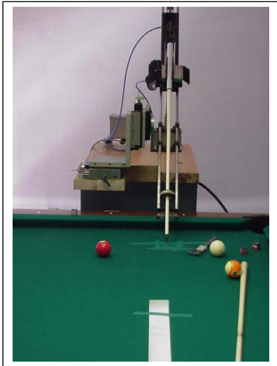
Figure 4. Jump-Cue Testing Machine Front View
