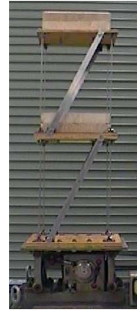
Figure 4.7 Braced Two Masses per Floor
