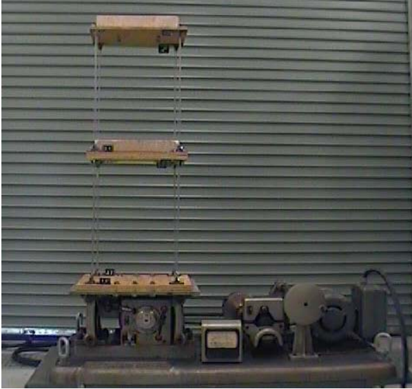
Figure 4.4 – Unbraced Structure with One Mass per Floor.
